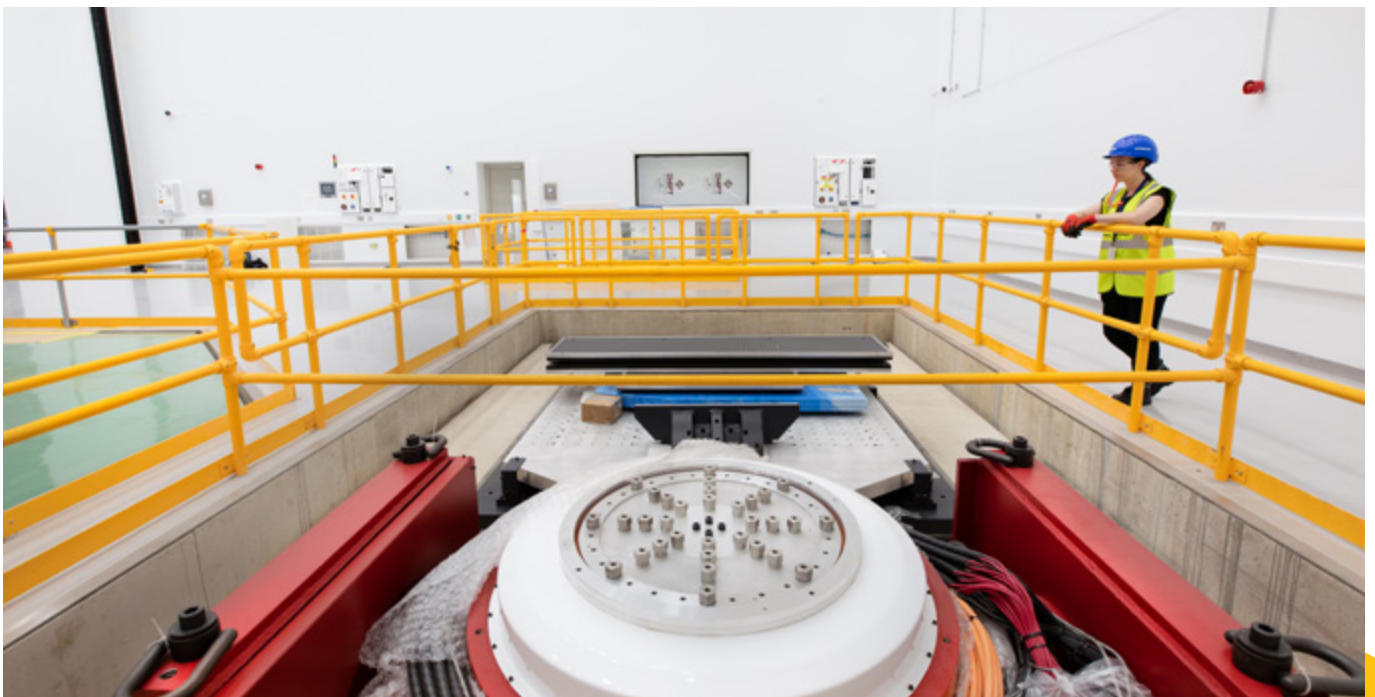
Vibration test equipment at the National Satellite Test Facility. Credit: STFC RAL Space
