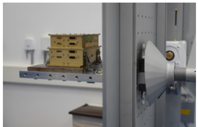
Pyroshock rig ready to test. Credit: STFC RAL Space
