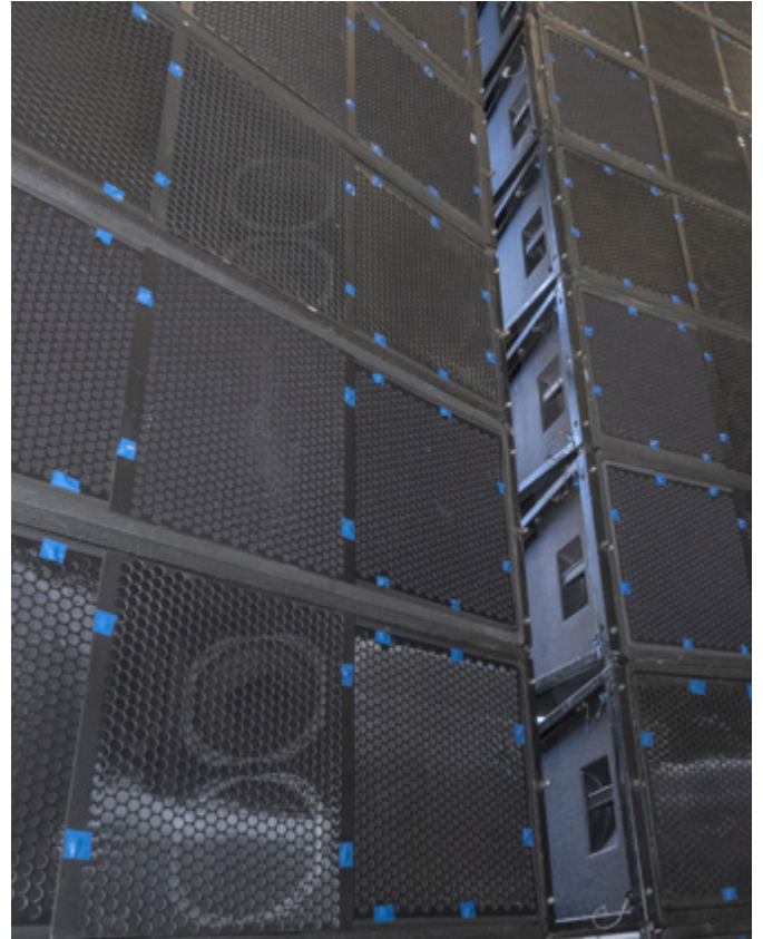
Direct field acoustic noise amplifiers. Credit: STFC RAL Space
